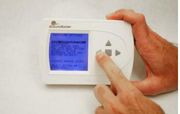
8. After the changes have been saved, the screen will return to the "Installer Settings" mode. Press the arrow left button to return to the main screen.
