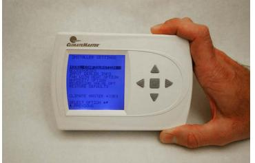
2. The "Installer Settings" menu will appear when the thermostat is in the correct mode.
