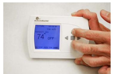
1. Make sure thermostat is in the "OFF" position. Hold the arrow up and arrow down keys for approx. 5 seconds to enter into the "Installer Settings" mode.
