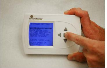
3. "Model Configuration" should already be highlighted. If so, press the center square button to select. If not, use the arrow up or arrow down keys to select this menu choice.
