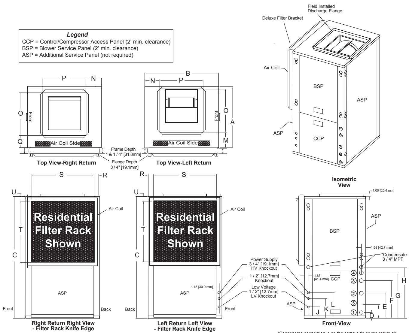
Note: Provide 2' minimum clear access to the Control/Compressor Access Panel and the Blower Service Panel.
