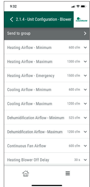
Airflow Configuration Screen on Mobile App
