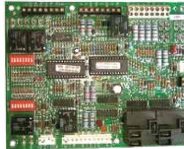
ClimateMaster’s enhanced DXM digital controls.
