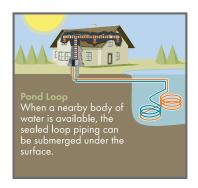
Pond Loops are usually very economical to install. If a pond or lake at least eight feet deep is available, pond loops can utilize the water (rather than soil) to transfer heat to and from the pond. A coiled pipe is placed in the water, which should cover about 1/2 acre.
