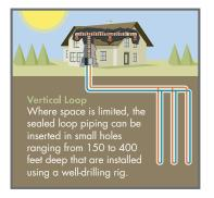
Vertical Loops are used extensively where land area is limited or soil conditions prohibit digging the more economical horizontal loops. A pair of pipes with a special U-Bend assembly at the bottom are inserted into a bore hole that averages between 150 to 250
