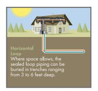
Horizontal Loops are installed in areas where the soil conditions allow for economical excavation. Taking up more land area than any other loop type, they are used where space permits. Trenches are normally about five foot deep with multiple pipes placed in the
