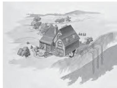
vertical bore. Bore hole depth ranges from 100-300 feet per system ton. Bores must be spaced from 10-15 feet apart and properly grouted. The land space required ranges from 100-200 square feet per system ton.
