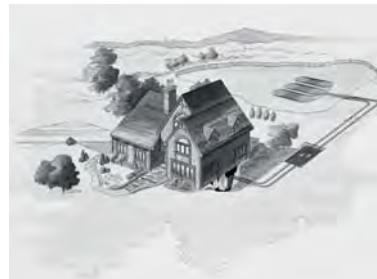
of the pond (lake). In most cases, 1/4 to 1/2 acre of water surface, with a minimum depth of 8-10 feet, is needed for a typical residence.
