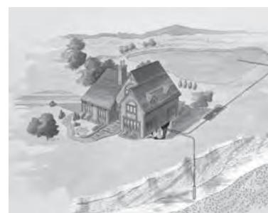
operation. Ditches, field tiles, ponds and streams are the most common discharge systems. Reinjection or semi-closed recirculation wells can also be utilized in some regions. In ideal conditions, an open loop application can be the most economical type of system to install.
