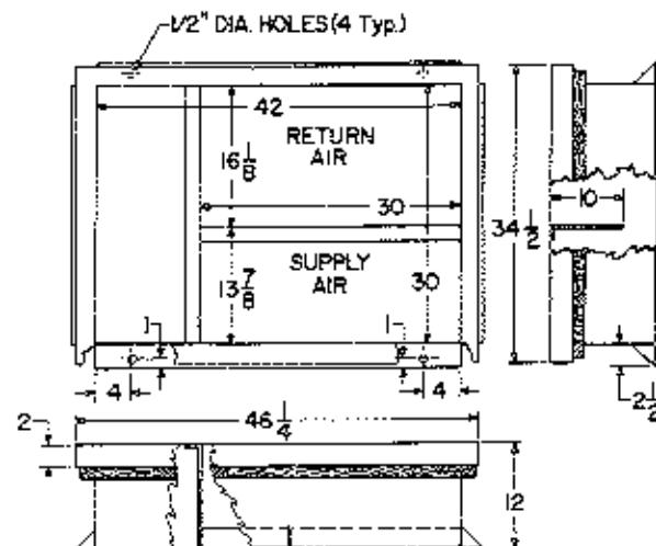
Shaded Area Indicate 3' Clearance must be left for access to Compressor and Electrical Panel.
