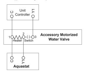
Figure 20: Accessory Motorized Water Valve -Typical Wiring Example #2
