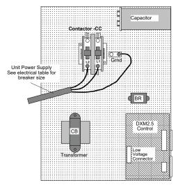
Note: 460V units with ECM, ClimaDry<sup>®</sup> II, or Internal Secondary Pump require a neutral wire.
