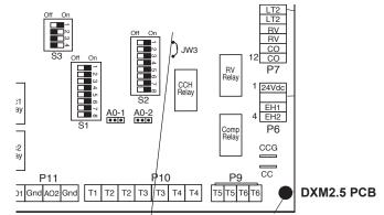
JW3-LT1 jumper should be clipped for low temperature operation. Do not clip JW3-LT1 in open-loop applications
