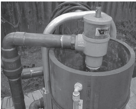
Figure 14a: Typical Cleanable Flush Cart Strainer (100 mesh [0.149 mm])
