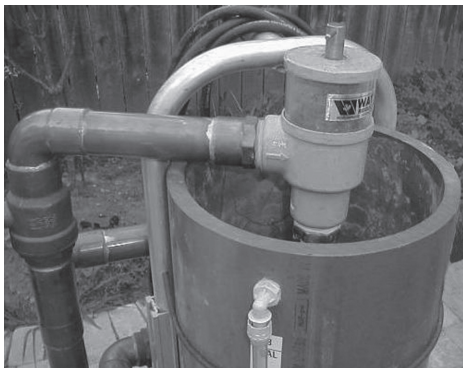
Figure 7a: Typical Cleanable Flush Cart Strainer (100 mesh [0.149 mm])
