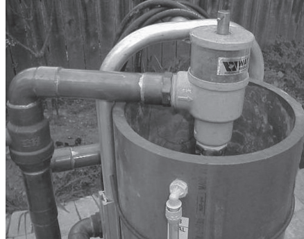
Figure 8b: Cam Fittings for Flush Cart Hoses
