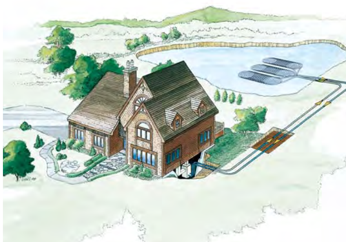
An example of a pond loop installation
