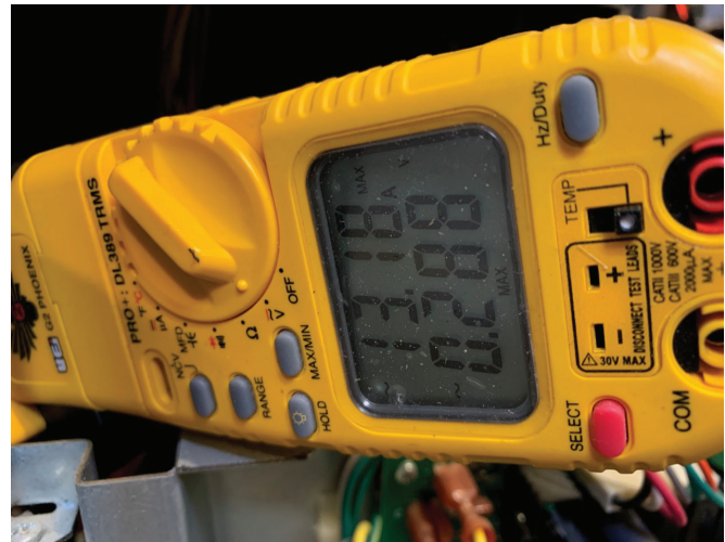
Inrush Current On a QE1860 13.18 amps on startup in cooling manual mode.
