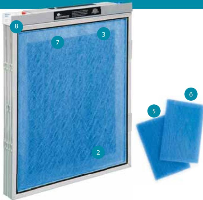
ClimateMaster's EarthPure® Polarized Media Electronic Air Cleaner installs directly into the 2"/1" filter rack of your ClimateMaster heat pump or air handler. The electronically enhanced media combines elements of both electronic and media air cleaners. Particles are electrically charged (polarized) and then collected in the high efficiency media. Polarized sub-micron particles join with other particles and are collected on subsequent passes.
