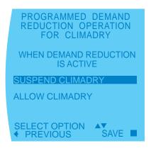
Adjust the Programmed Demand Reduction Climadry™ settings using the up/down arrow buttons. Press the center button to save changes.
