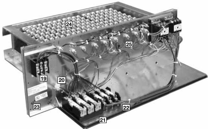
Power hook-up in the field is easy with single-point wiring to a terminal block ([19]) and a polarized plug for the low-voltage connection ([20]). The electric furnace comes with fuses for the unit ([21]) and for the electric furnace ([22]), and is UL certified ([23]). The electric heating elements are of a wound-wire construction ([24]) and isolated with ceramic bushings. The limit switch ([25]) protects the design from over-temperature conditions.
