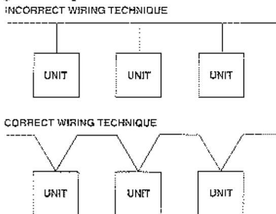
3. Do not use wire nut devices for connecting communication cable.
