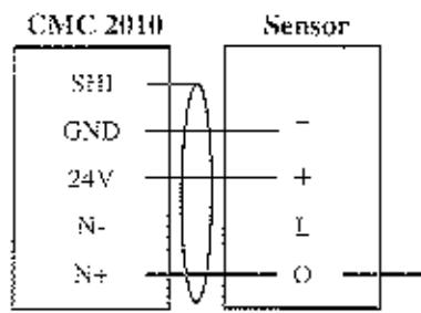
Connected to "L" terminal on CMC
