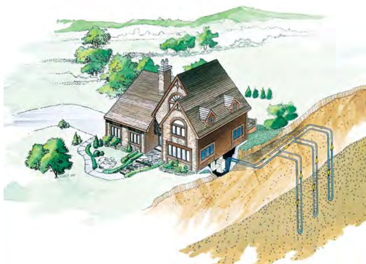
An example of a vertical loop installation
