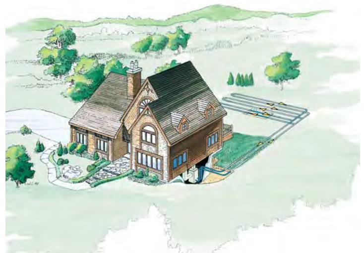
An example of a horizontal loop installation
