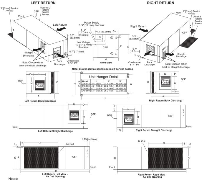
1. While clear access to all removable panels is not required, installer should take care to comply with all building codes and allow adequate clearance for future field service.
