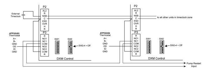
Digital Night Setback and Pump Restart Wiring Connections - UNITS Note: Can connect all heat pumps to one timeclock.
