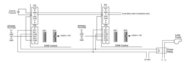
Digital Night Setback and Pump Restart Wiring Connections - UNITS Note: Can connect all heat pumps to one timeclock.
