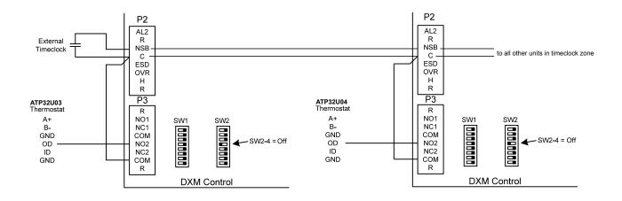
Digital Night Setback Wiring Connections - UNITS Note: Can connect all heat pumps to one timeclock
