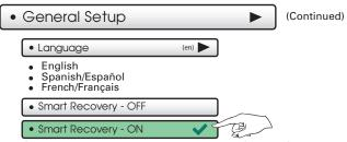
Smart Recovery turns on the heat or cool before the Occupied start time to bring the room temperature to the Occupied setpoint at the start of the Occupied time period. Please allow 4-8 days for Smart Recovery time to adjust. When used with a heat pump, electric strip heat will be disabled while Smart Recovery is active.
