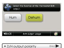
The D/H Output polarity may be set for Normally Open or Normally Closed to accommodate different types of humidification and dehumidification equipment.
