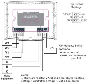
2) Connect the normally open Condensate Overflow switch between the two SENSOR terminals. To enable the function, set MENU > Settings > Installation Settings > Sensor Settings > AUX IN use to Condensate Overflow. When triggered, cooling is turned off. If the switch opens, cooling will resume, and a condensate pan overflow alert will be triggered to notify the user that servicing of the condensate drain is required.
