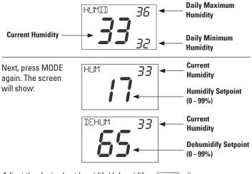
Adjust the desired set humidify/dehumidify value with UP or DOWN buttons
