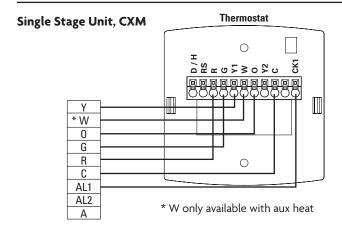
Note: Do not clip jumper JW1 on CXM board
