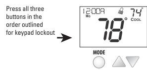
To **unlock** the keypad, press and hold the MODE button. While holding the MODE button, press the UP and DOWN buttons together for 2 seconds.
