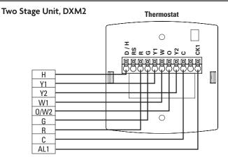
If using the integral condensate overflow sensing in the heatpump, an overflow condition generates a FAULT signal which halts equipment operation. Bringing that signal into CK1 and setting DRY CONTACT USE (setup step #29) to FDD will show EQUIP FAULT on the display.
