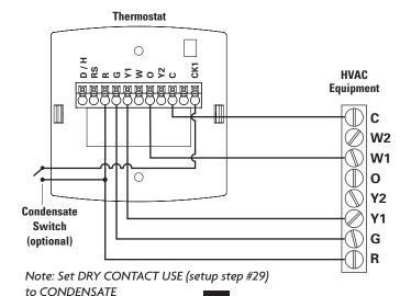
2 Stage Heat, 2 Stage Cool with wired remote sensor
