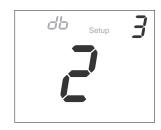
Adjust the minimum difference between cooling & heating setpoints by pressing the **UP** and **DOWN** buttons.
