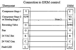
Note 1: Optional connection for Heating Stage 2 operation. Thermostat "Y2" option must be configured as
