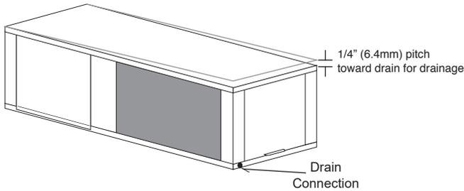
**Figure 3: Typical Horizontal Unit Installation**
