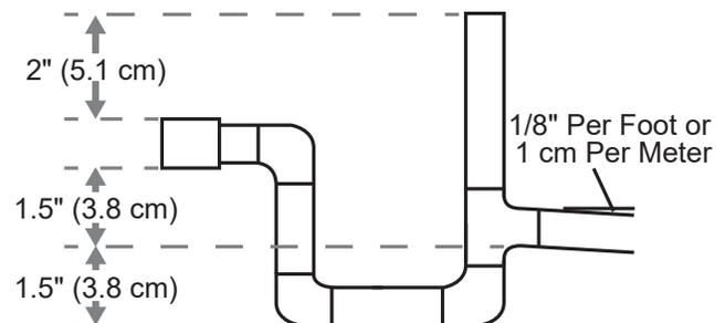
**Figure 10c: Vertical Internal Condensate Trap**
