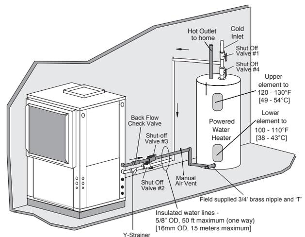
**Figure 15: HWG Double Tank Installation**
