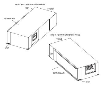
**Horizontal Units Condensate Piping** - Pitch the unit toward the drain as shown in Figure 2 to improve the condensate drainage. Ensure that unit pitch does not cause condensate leaks inside the cabinet.
