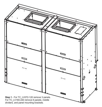
**Step 1** - Remove control box access panel and panel box will be relocated to.
