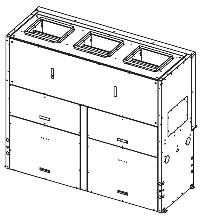
**Step 1** - Remove 5 panels, dividers, and panel mount brackets.
