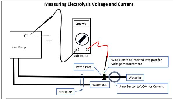
Measure the electrolysis voltage using a volt meter between the heat pump ground and a #14 AWG solid copper wire electrode inserted into the water using a Pete's style access port.
