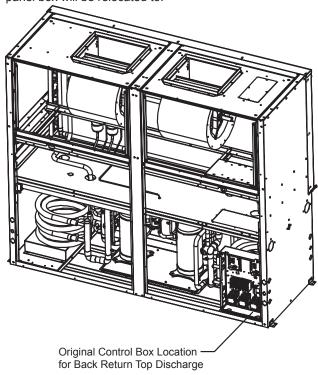
**Step 2:** Unattach all wires from components, remove the control box, tag wires. Pull wires out of box.
