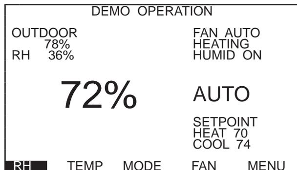
The starting mode (heating or cooling) depends on the loop temperature at the time when Demo Mode is entered. The unit will operate in heating or cooling based upon the following algorithm.
