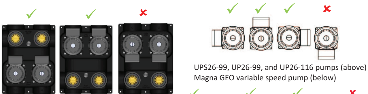
Figure 5b: Acceptable terminal box locations
