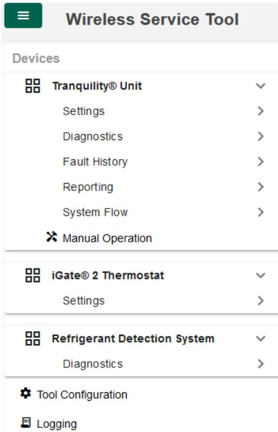
The product connected to the WST determines the options that display in the Home screen. For example, Refrigerant Detection System does not display in the WST Web App if an RDS is not detected. The following examples illustrate Home screen behavior based on the connected product.
