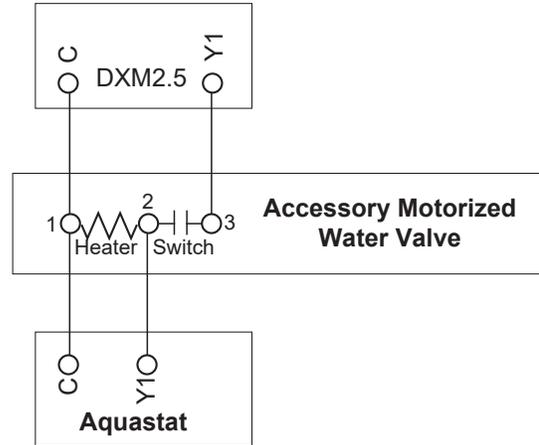
**Figure 8: Accessory Motorized Water Valve - Typical Wiring Example #2**
