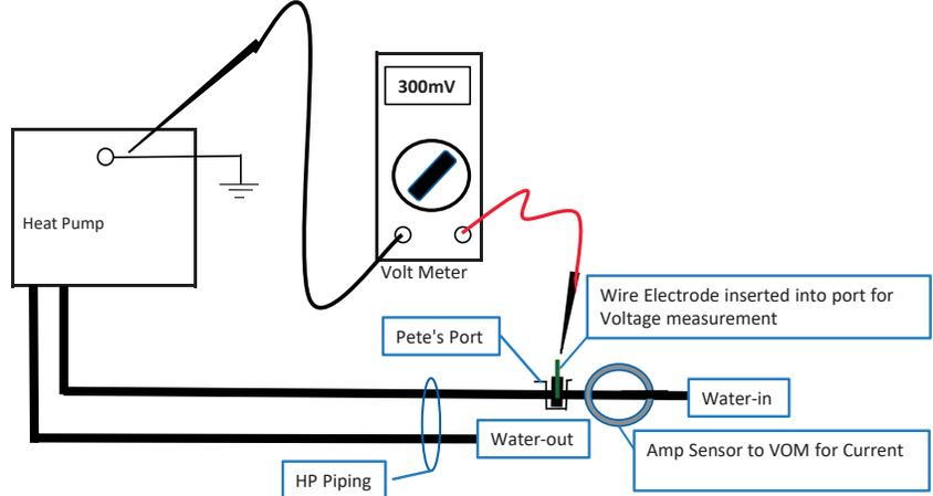
Measure the electrolysis voltage using a volt meter between the heat pump ground and a #14 AWG solid copper wire electrode inserted into the water using a Pete's style access port.
