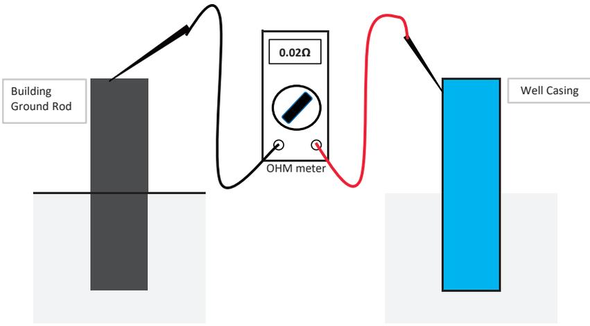
Measure the earth ground bond using an Ohm meter between the building's ground rod and the steel well casing.
