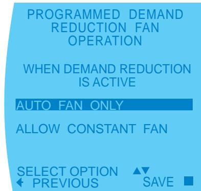
Adjust the Programmed Demand Reduction Fan settings using the up/down arrow buttons. Press the center button to save changes.
