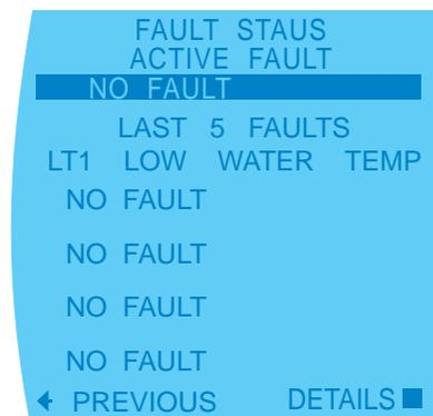
Navigate between system fault codes using the up/down arrow buttons. Press the center button to view more information about potential reasons why the highlighted fault may have occurred.
