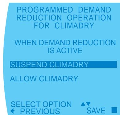
Adjust the Programmed Demand Reduction Climadry™ settings using the up/down arrow buttons. Press the center button to save changes.
