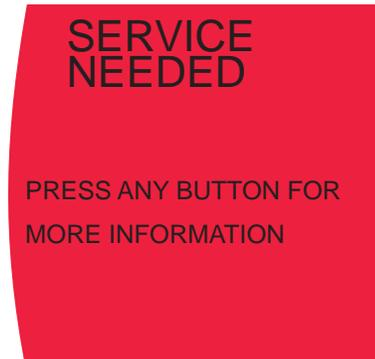
The next screen will display the model and serial number of your ClimateMaster unit, the phone number of your installing contractor, and the fault code and a description of the fault that triggered the Service Needed screen.
