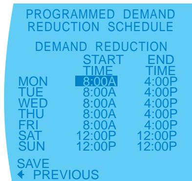
Adjust the Programmed Demand Reduction Schedule start and end time settings using the up/down arrow buttons in increments of 10 minutes. Press the center button to save changes.
